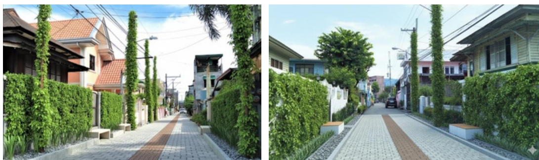
Figure 6 to 7. Reimagined poblacion streets with permeable pavement, vertical garden, and rain gardens along curblines.
