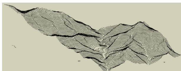
Figure 3. Digital Terrain model from Drone survey.
